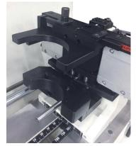
gasket surface so valve seats are machined to the same equal depth, head after head.
