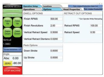
Dwell and Retract are the important settings that allow precision valve seat machining for features such as surface finish and CONCEN.
