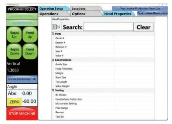
Information and Specifications can be saved together with the programs for each cylinder head. All programs can be backed up for security.
